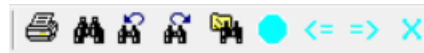
Figure 5.6-1 toolbar, print, find Print, print or output PDF document Find to find in the current document Find previous Find next Find in files to find in multiple documents Toggle bookmark to mark the current line Goto prev bookmark to find the previous tag Goto next bookmark to find the next tag
